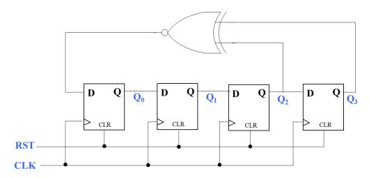
Write a Verilog program that implements the LFSR according to the circuit above. Simulate / work out the operation of the circuit to work out the bit sequence of Q.
